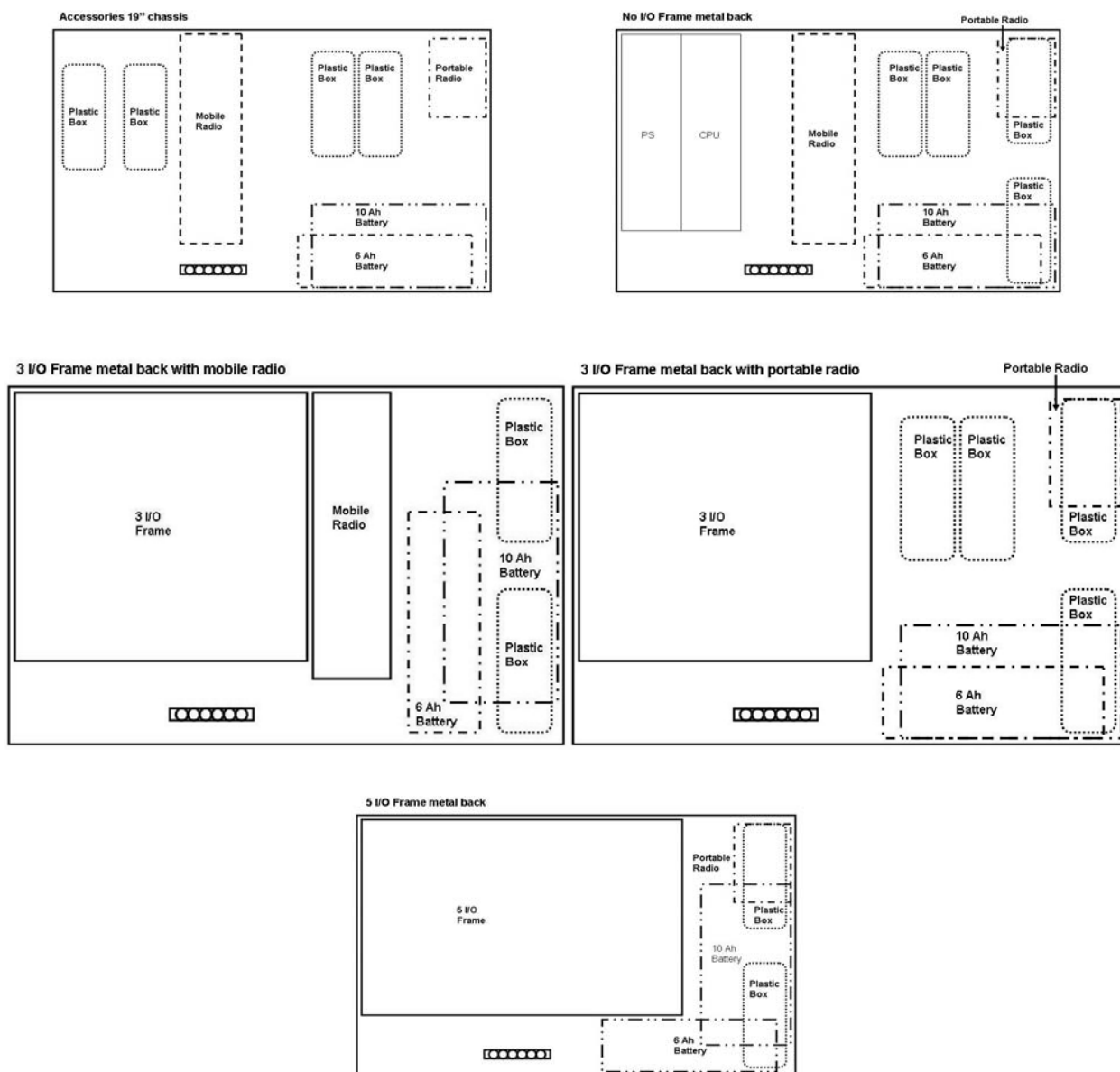
Figure 2-28 19" Frame Metal Back Installation Combinations
