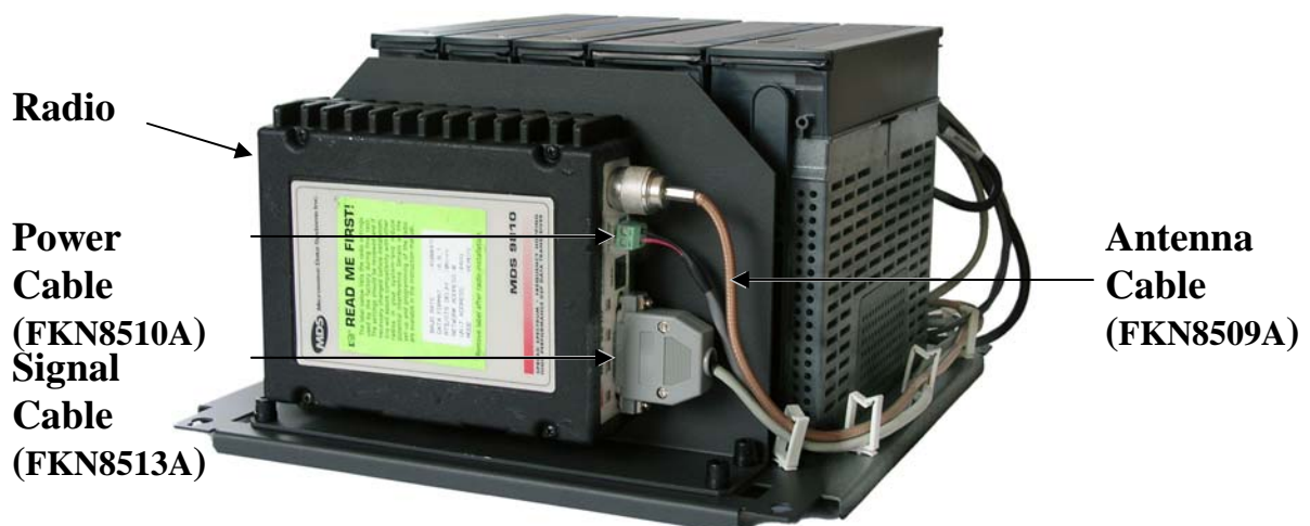
Figure 21-59 MDS Radio Modem Installed on ACE3600 Chassis – Cable Connections
