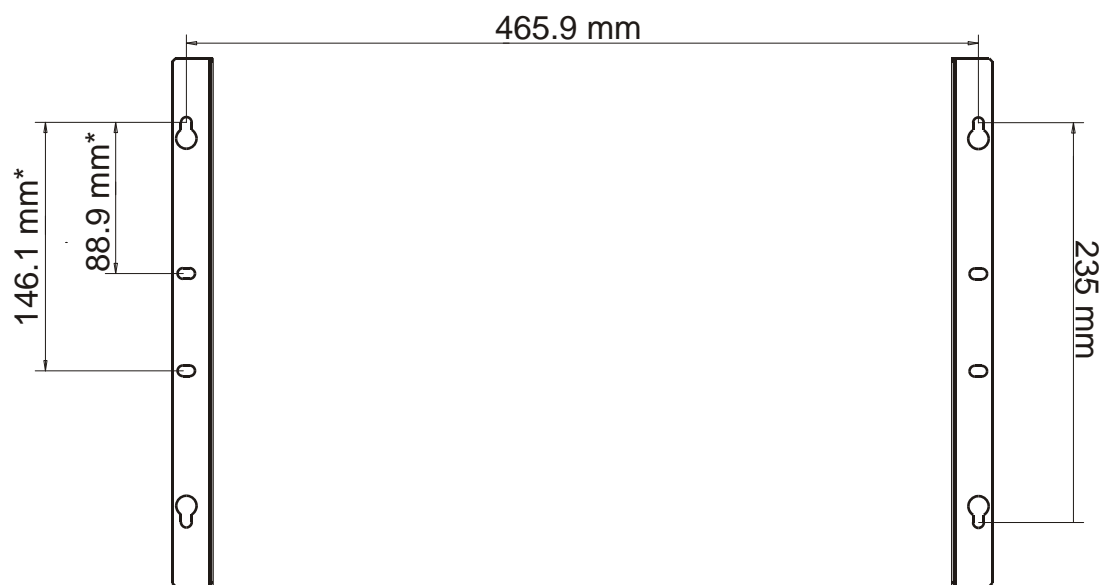
Figure 2-10 8 I/O Frame (19") Metal Back Installation Dimensions
