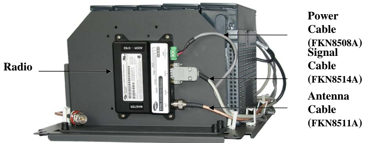
Figure 21-48 TransNET 900 Radio Modem Installed on ACE3600 Chassis – Cable Connections
