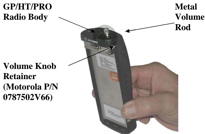
Figure 21-30 Attach Retainer to Radio
