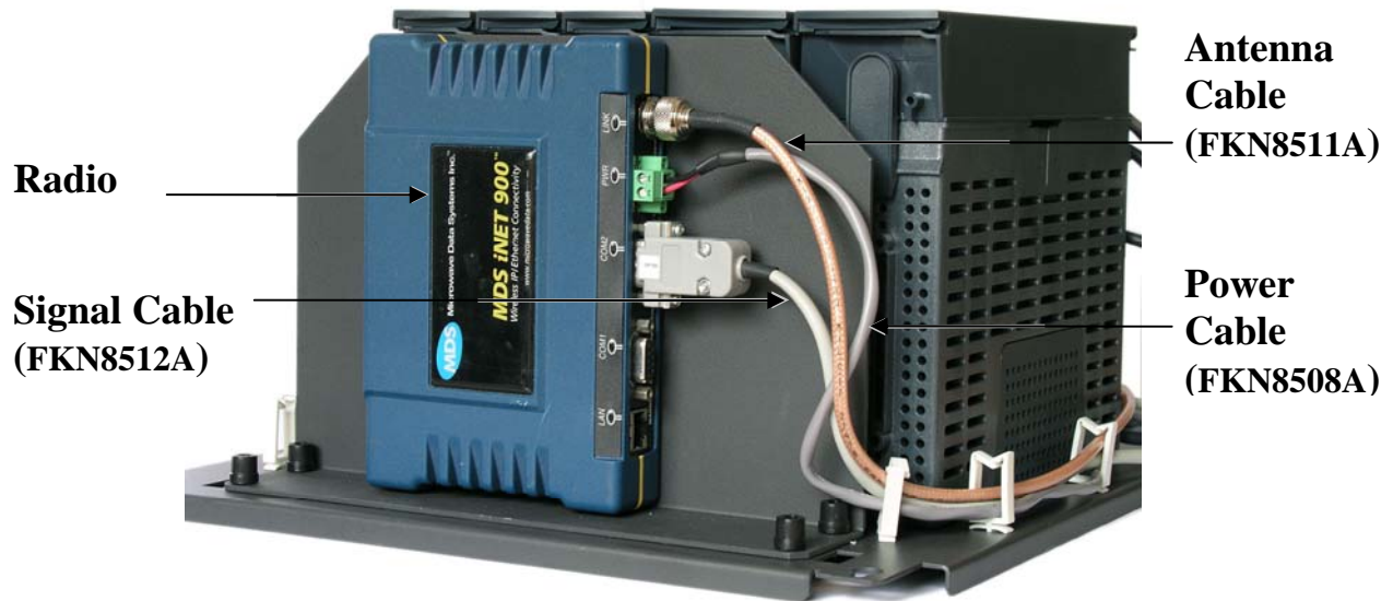
Figure 21-53 iNET 900 Radio Modem Installed on ACE3600 Chassis – Cable Connections
