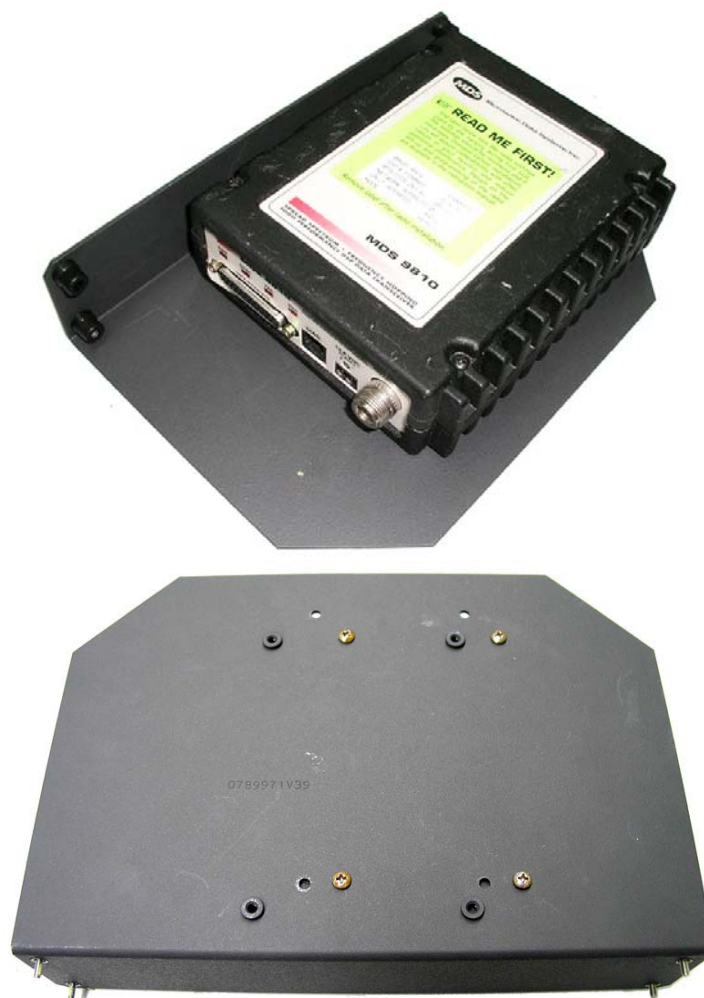
Figure 21-57 MDS Radio Mounted on Metal Bracket - Front and Rear View
